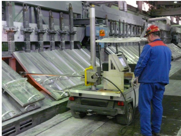
Figure 4.11 Bath and Liquidus Temperature Measurements at Aldel
