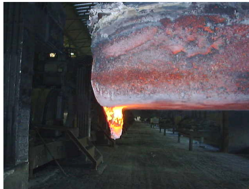
Figure 2.18 Example of an Anode Spike at Voerdal
