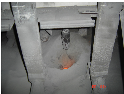
Figure 4.10 Point Feed Hole for Alumina Feeding at Aldel
