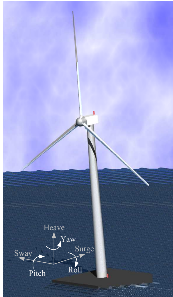
Figure 1.2: The floating platform's 6 DOFs
