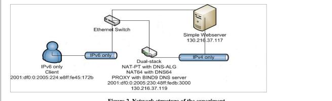
Figure 2. Network structure of the experiment
