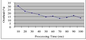
Figure 2 The Overheads of the ServiceHub
