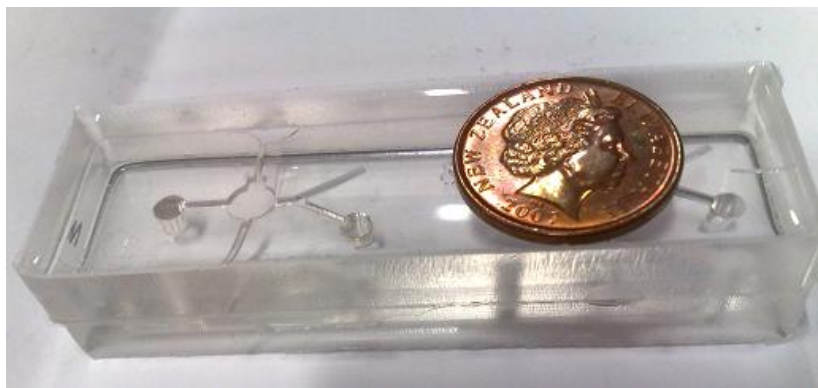
Figure 3.3. PDMS based microfluidic chip with the inlet and outlet. The depth of the channel was 1 mm.
