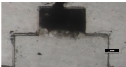
Figure 7.17. Chemically prepared PPy hydrogel composite.
