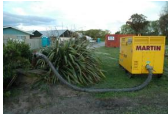
Photo 8.4: Application of series of mobile pumps in severely damaged region (Kaiapoi 24 September 2010) (Source: Author's own)
