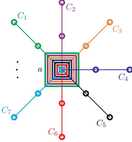
FIG. 2. (Color online) Greechie orthogonality diagram with an overlaid value assignment reflecting the proof of Theorem 9 associated with the configuration of contexts  $S_a = \{C \mid C \in \mathcal{C} \text{ and } a \in C\} \subseteq \mathcal{C}$ . Different contexts  $C_i$  are drawn in different colours.
