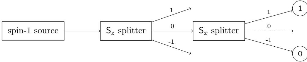
FIG. 5. Experimental setup of a configuration of quantum observables rendering random bits certified by quantum value indefiniteness.
