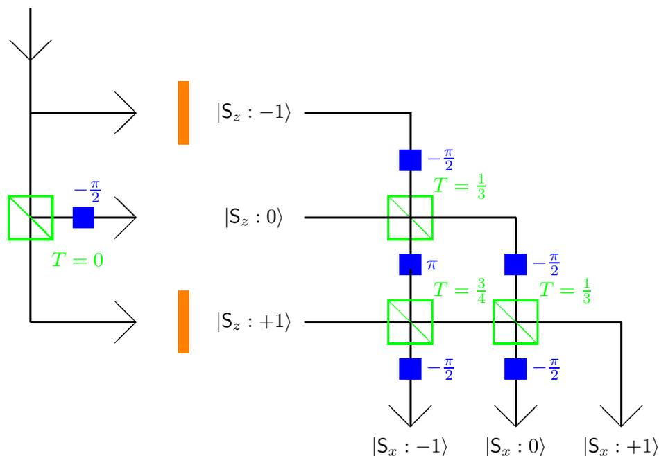
FIG. 6. (Color online) Configuration of a random number generator with a preparation and a measurement stage, including filters blocking  $|S_z : -1\rangle$  and  $|S_z : +1\rangle$ . (For ideal beam-splitters, these filters would not be required.) The measurement stage (right array) realises a unitary quantum gate  $U_x$ , corresponding to the projectors onto the  $S_x$  state observables for spin state measurements along the  $x$ -axis, in terms of generalised beam-splitters..
