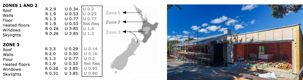
Figure 1, Timber framed house insulation requirements of NZ Building Code compared to PH values Figure 2, NZ’s first PH in Auckland, certified in October 2012 (courtesy of Carters)
