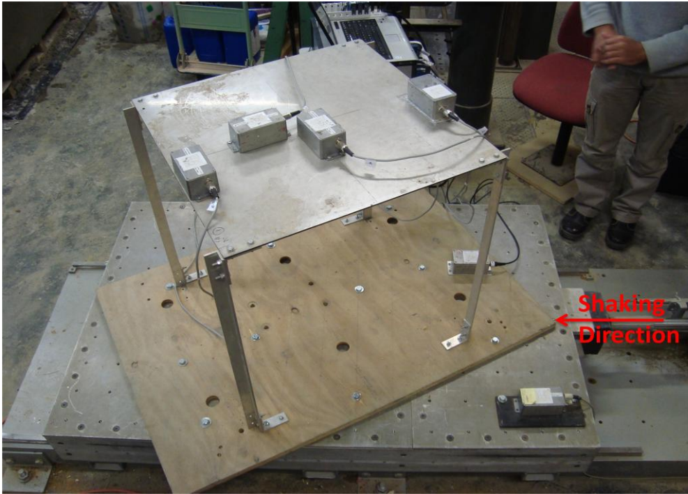
Figure 4.1 Laboratory structure fitted on the shake table at an angle of 20 degrees to the direction of shaking
