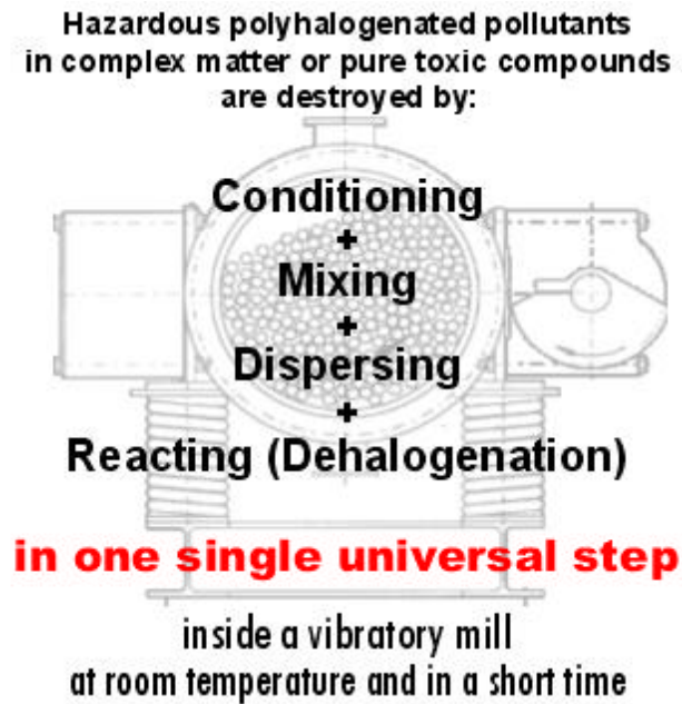
Figure 38. Overview of the ball milling process as defined by a technology vendor. Simplicity and the ability to turn toxic substances into harmless products is emphasised (Birke 2001).
