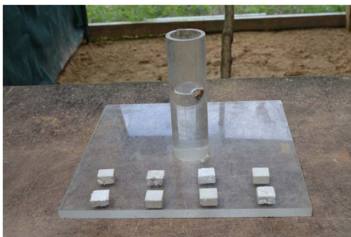
Figure 5. Sinking vs. floating experimental set up. doi:10.1371/journal.pone.0103049.g005
