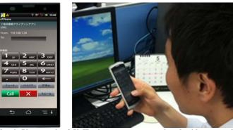
Fig. 4. Photograph of VoIP phone prototype equipped with proposed AEC method.
