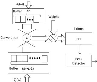
Fig. 3. Delay Estimation by MDF-GCC.
