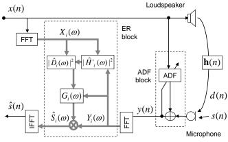
Fig. 1. Block diagram depicting conventional AEC method
