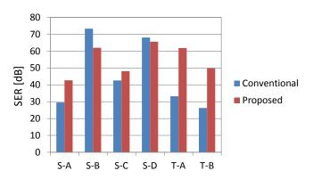
Fig. 9. Comparison of echo reduction performance by SER (single talk with office noise at 15 dB SNR).
