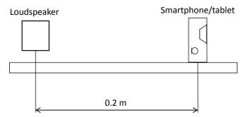
Fig. 6. Test arrangements for objective measurements.
