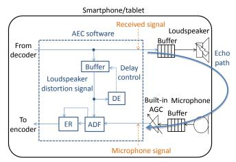
Fig. 2. Block diagram depicting proposed AEC method developed for smartphone and tablet devices.
