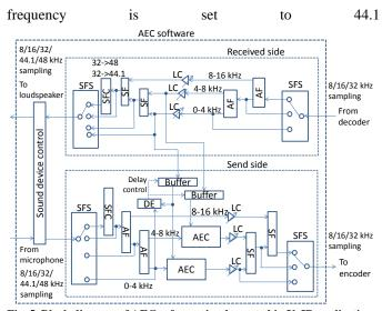
Fig. 5. Block diagram of AEC software implemented in VoIP application.
