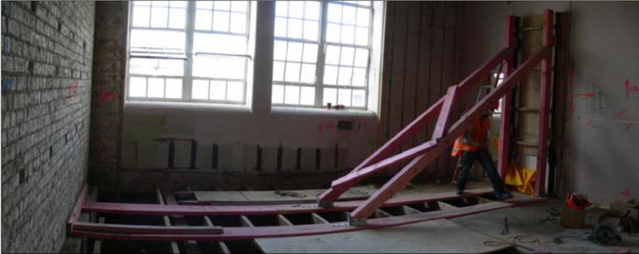
Figure 4: Out-of-plane test setup
