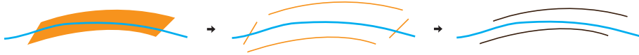
Fig. 5. Extract approximately parallel arcs. Left: A given user stroke and a unit. Middle: We cut the outline of the unit into four candidate arcs according to extreme points and corner points. Right: We detect two arcs that are approximately parallel to the user stroke.
