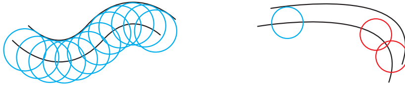
Fig. 3. Arc parallelism. Left: An arc, congruent circles centred on this arc, and an envelope parallel to the given arc. Right: Two arcs defined by a translation of one arc into the other; those two arcs are not parallel.
