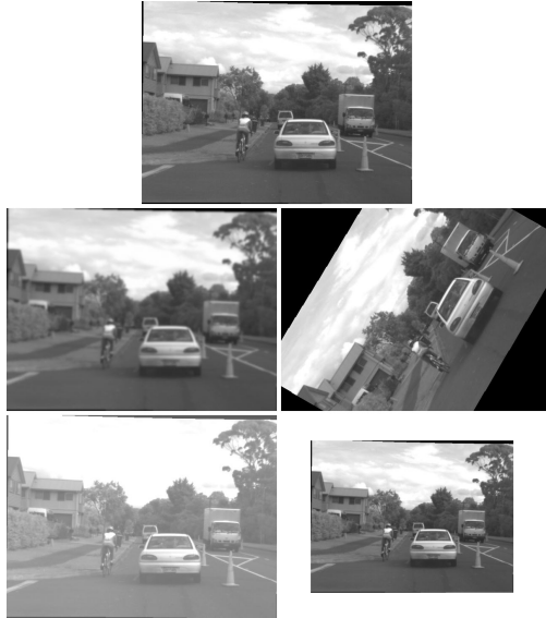
Fig. 1. Sample of an image of the discussed video sequence ( top , the black pixels at the border are due to rectification of the stereo frames), with four images after processing, illustrating blurring ( middle, left ), rotation ( middle, right ), brightness changes ( bottom, left ), and scaling ( bottom, right ). The used sequence of 400 stereo frames is in Set 4 of EISATS [5], and called “Cyclist”; 640 \times 480 images are recorded with 10 bit per pixel.
