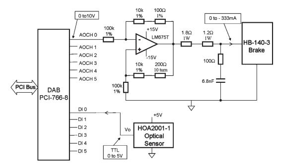
Fig. 6. Interface electronics between the DAB and one of the exercise stations.
