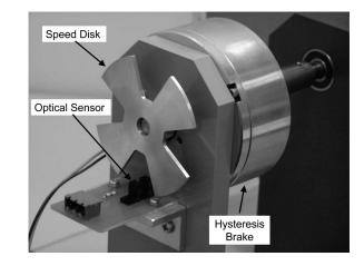
Fig. 5. Optical sensor used for movement and speed measurement.
