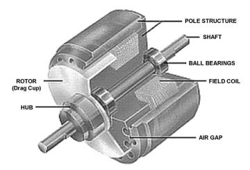
Fig. 1. Internal structure of a hysteresis brake (reproduced from Magtrol Inc. [5]).
