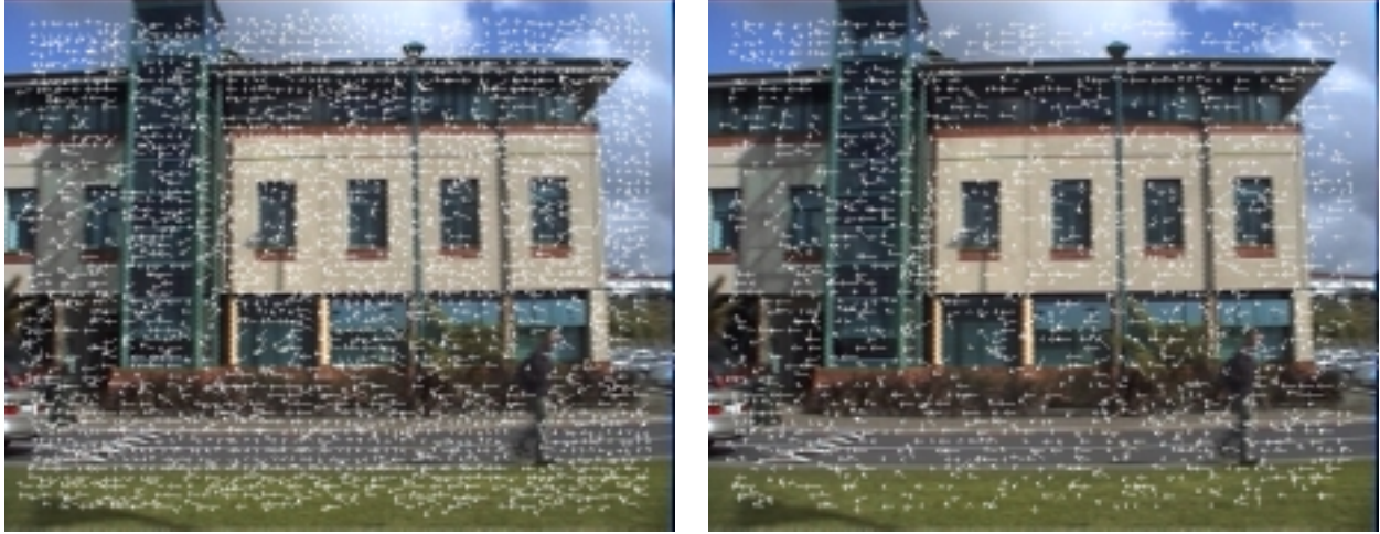
Figure 6. (Left) Colour Horn and Schunck flow with \alpha = 3 and (Right) colour Barron and Klette flow with \beta = 1.0 , both with post-thresholding of \|\nabla I\|_2 > 5.0 and 100 iterations.
