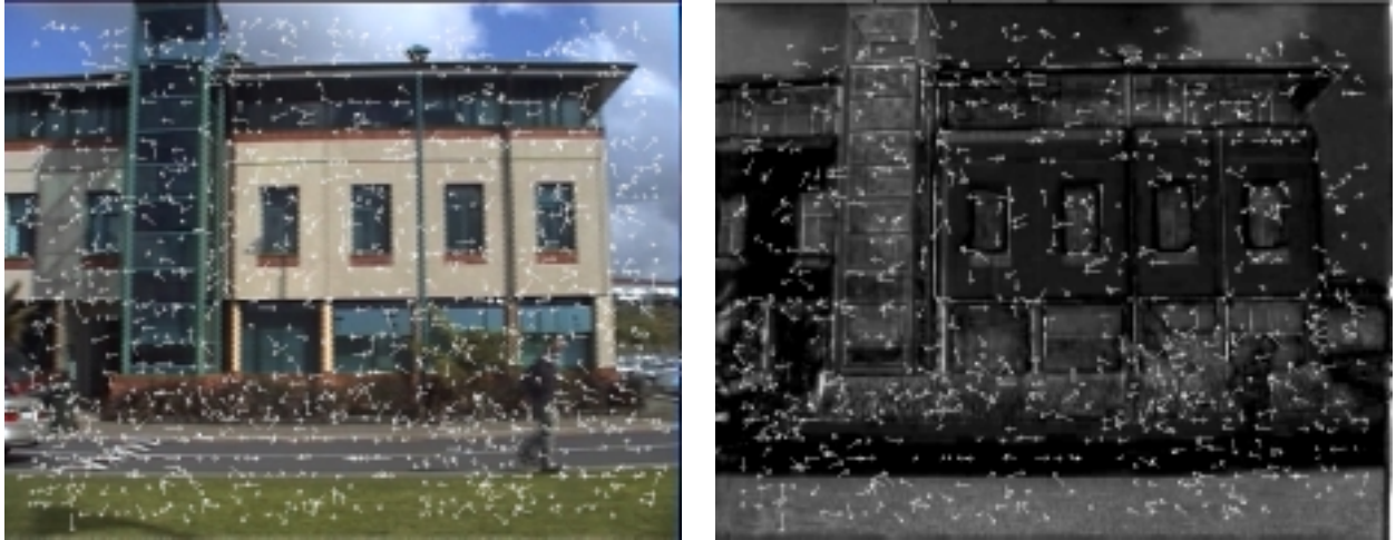
Figure 5. (Left) Colour Ohta flow and (Right) saturation/Y Ohta flow, both with post-thresholding of \|\nabla I\|_2 > 5.0 .
