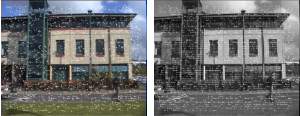
Figure 7. (Left) Barron and Klette flow for the Y and saturation images and (Right) Barron and Klette flow for the Y image only, both with post-thresholding of \|\nabla I\|_2 > 5.0 and 100 iterations and \beta = 1.0 .
