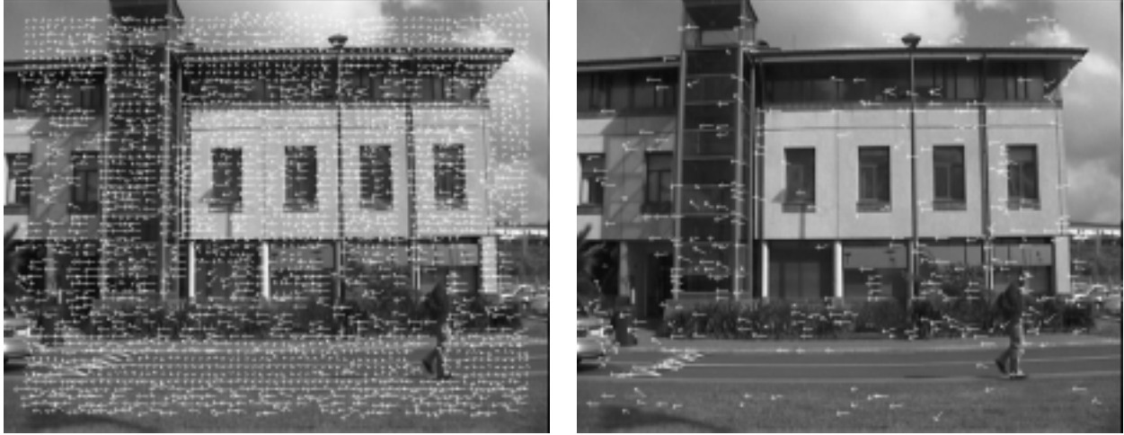
Figure 2. (Left) The Horn and Schunck flow for the Y image with \alpha = 3 and 100 iterations and post-thresholding of \|\nabla I\|_2 > 5.0 and (Right) the Lucas and Kanade for for the Y image with smallest eigenvalue thresholding of \tau > 5.0 .
