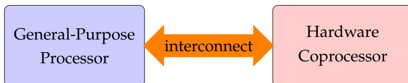
Figure 1.6: Typical hybrid hardware acceleration system.
