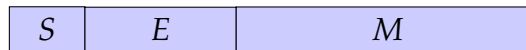
Figure 1.12: IEEE-754 floating point format ( S represents a sign bit, E represents an exponent field, and M is the mantissa field).
