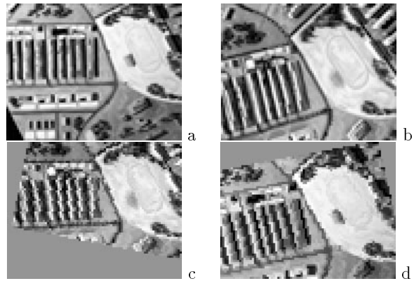
Figure 14. [11] Matching of images M11 (a) and M19 (b) from the RADIUS-M set: the affinely transformed images M19 (c) and M11 (d) yield the best least-square correlation found (0.68 and 0.82, respectively).
