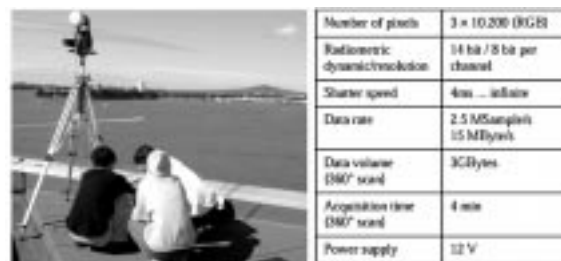
Figure 3. EYESCAN camera and [32] its basic parameters.
