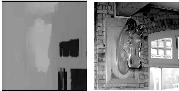
Figure 18. SDPS reconstruction of the “Horse” scene: the grey-coded range (DEM) image (left) and the corresponding cyclopean image (right) formed by fusing images of the stereo pair in line with the DEM.
