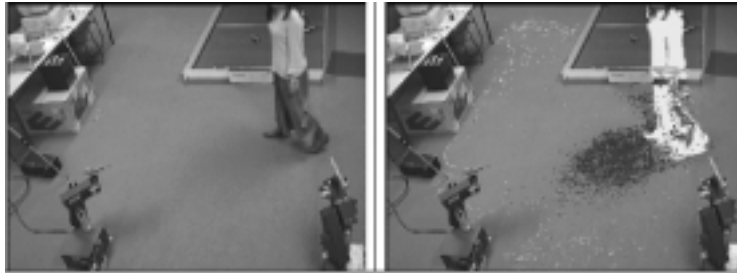
Fig. 3. Background subtraction for uniform lighting: left - the original frame, right - the result after background subtraction.
