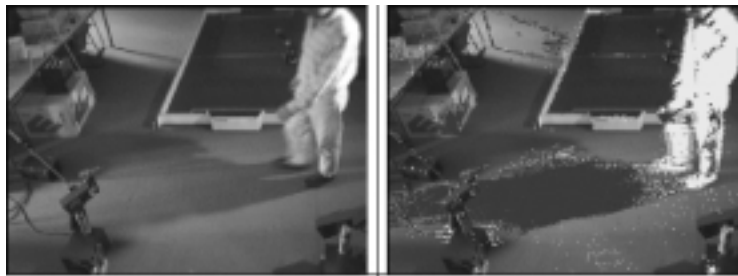
Fig. 9. Here, starting with static frames (i.e. without moving people) we continue with 5 frames showing moving people until the current frame: left - the current frame, right - the result after background subtraction.
