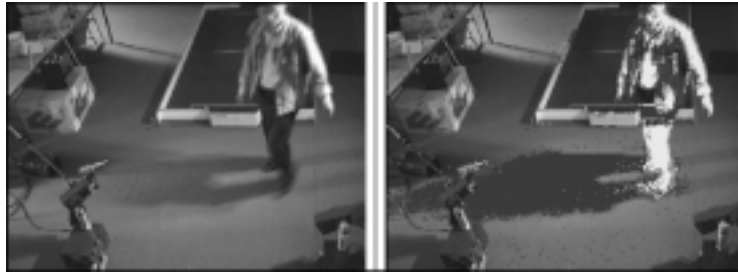
Fig. 7. Background subtraction for lighting coming from window plus two extra lights: left - the original frame, right - the result after background subtraction.
