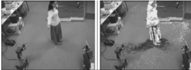
Fig. 4. Background subtraction for uniform lighting plus one extra light: left - the original frame, right - the result after background subtraction.
