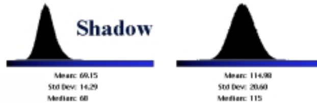
Fig. 1. Value distribution in the Blue channel of a region of the background: left - with shadow, right - without. This shows a typical situation: shadow means reduced intensity and reduced ‘dynamics’.
