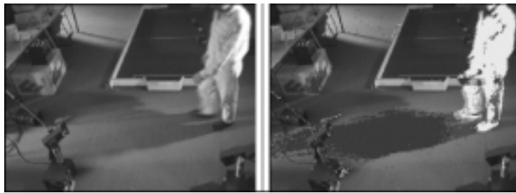
Fig. 6. Background subtraction for lighting coming from window plus one extra light: left - the original frame, right - the result after background subtraction.
