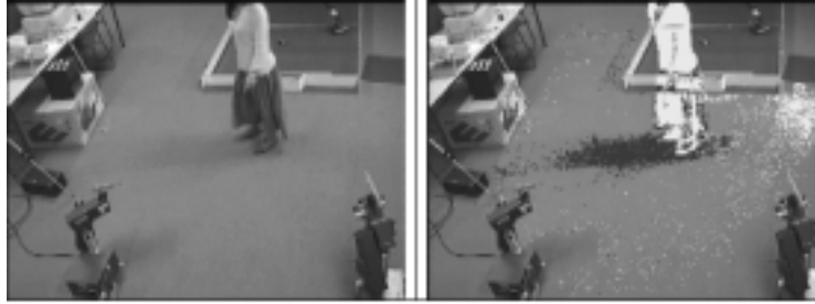
Fig. 5. Background subtraction for uniform lighting plus two extra lights: left - the original frame, right - the result after background subtraction.
