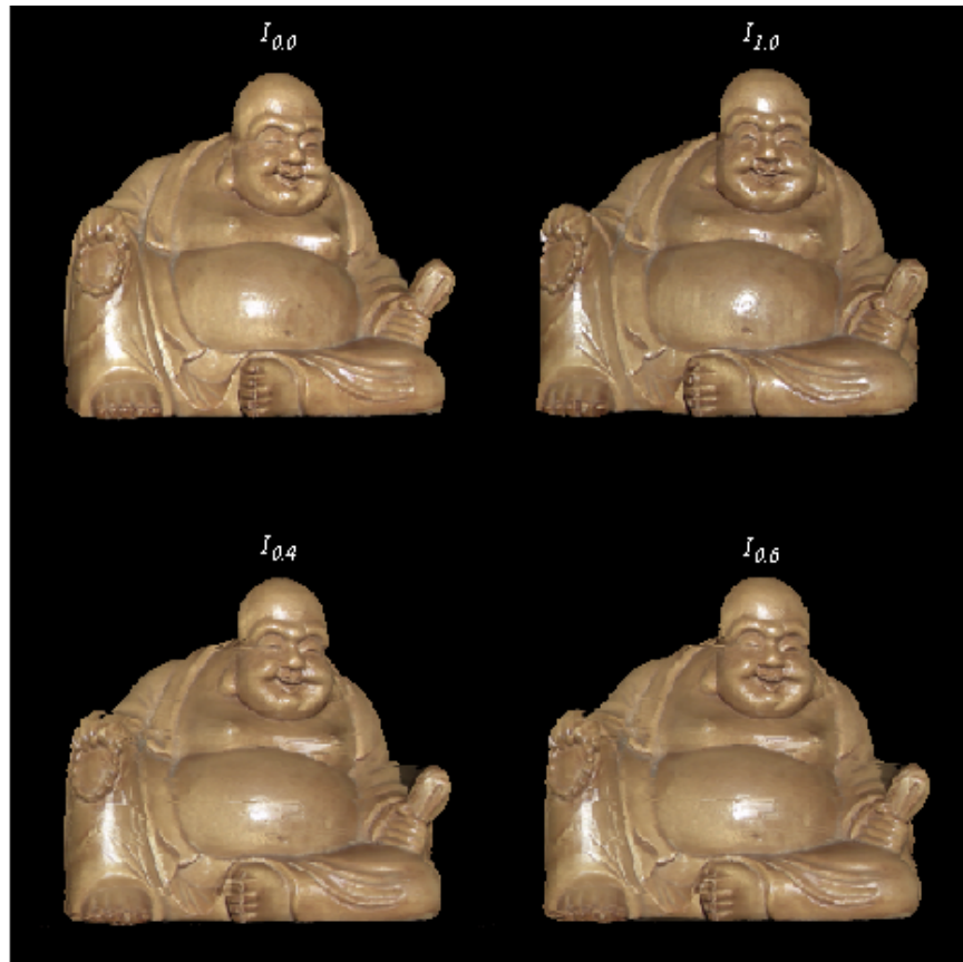
Figure 16: The result of synthetic views, I_{0.4} and I_{0.6} , are generated from two original Buddha views, I_{0.0} and I_{1.0} , with rotation angle 20 degrees.
