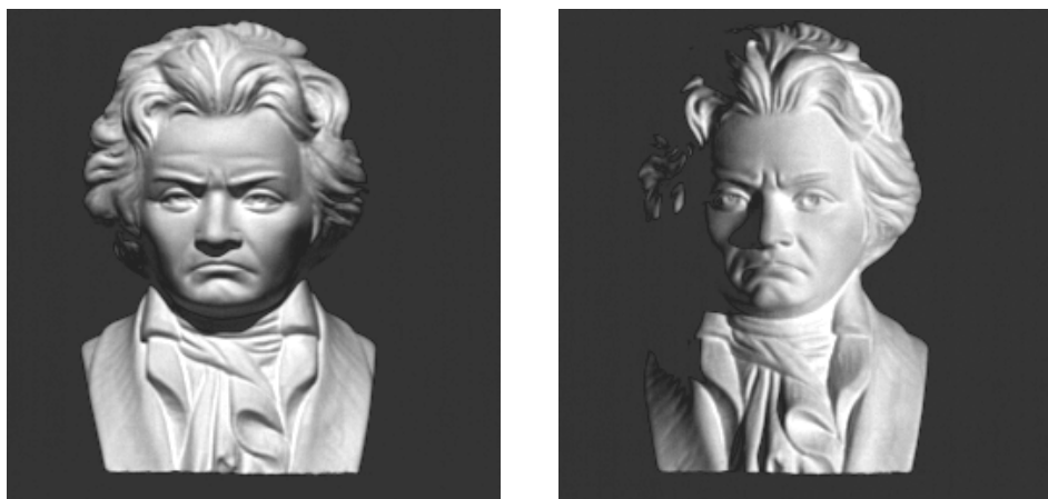
Figure 7: Two irradiance images of a real Beethoven plaster statue, both light sources generate self-shadows and cast-shadows in the images
