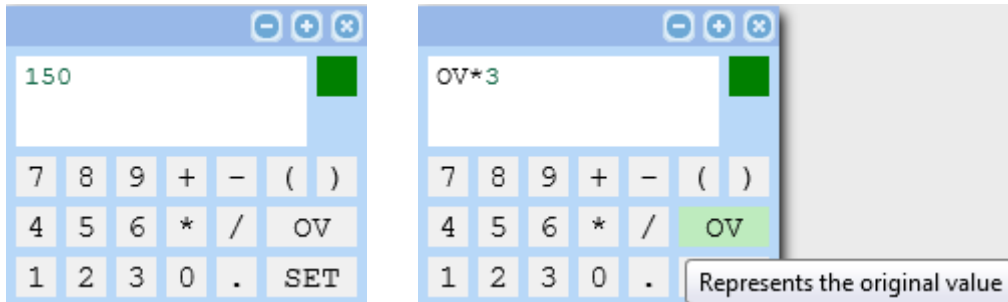
Figure 5.76: Two examples of the Numeric Value Interface. Left: Assigning a specific value of 150. Right: Modifying the OV (Original Value), the mouse is over the OV button, highlighting it and displaying the tooltip (if defined).
