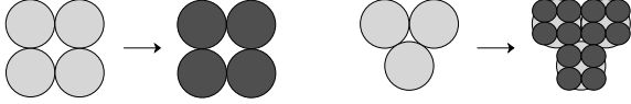
Figure 2: Mappings of orthogonal (on the left) or hexagonal (on the right) grids into an orthogonal grid.
