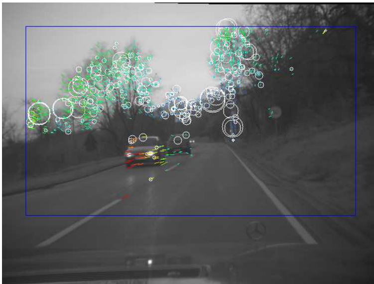
Fig. 9. Tracked points and detected scales (defining the size of the shown disks).
