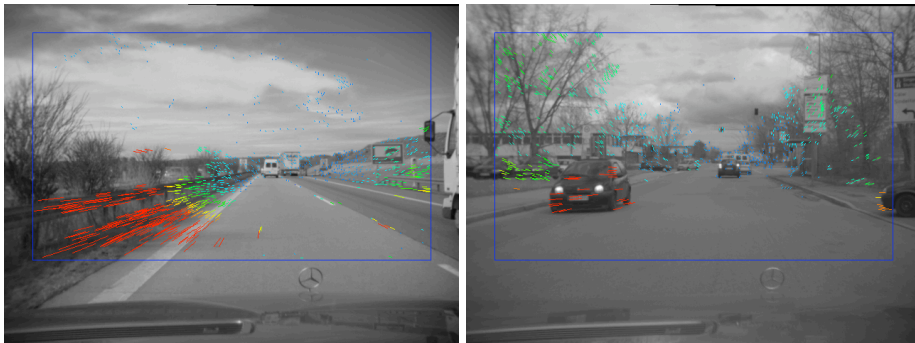
Fig. 3. Optical flow computed for Sequences 1 and 2.
