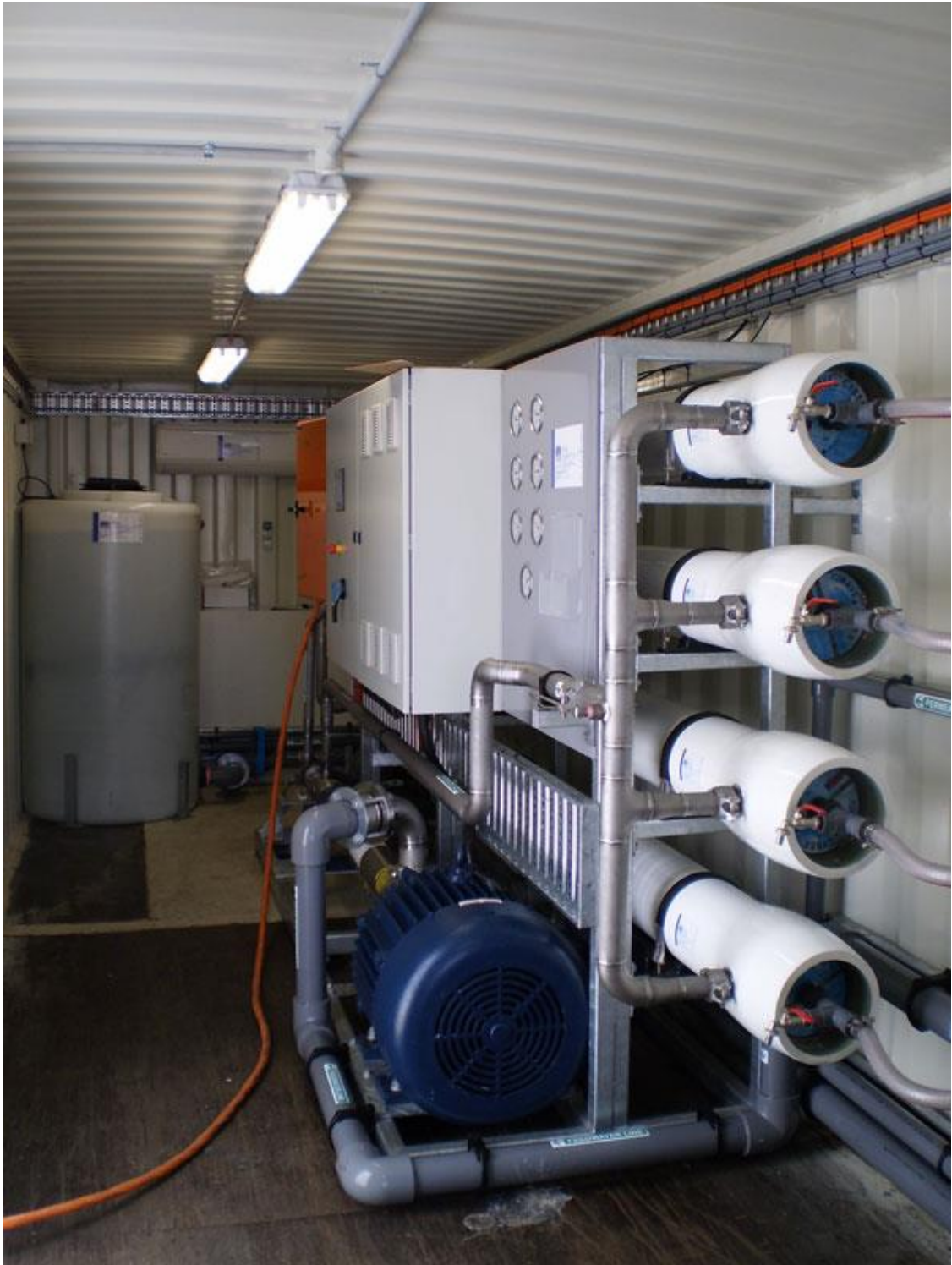
Figure 6.9. A Photograph of a Commercial 500m 3 /day SWRO plant housed in a Sea Container (MakWater, 2014).
