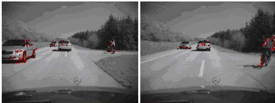
Fig. 5. 6D vision result, showing only moving object points which are not classified as being static background. Clustering of the shown dots allows identification of those three cars and of the bicyclist.
