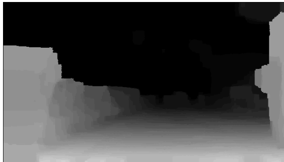
Fig. 3. Edge detection followed by belief-propagation allows to calculate this dense depth map.
