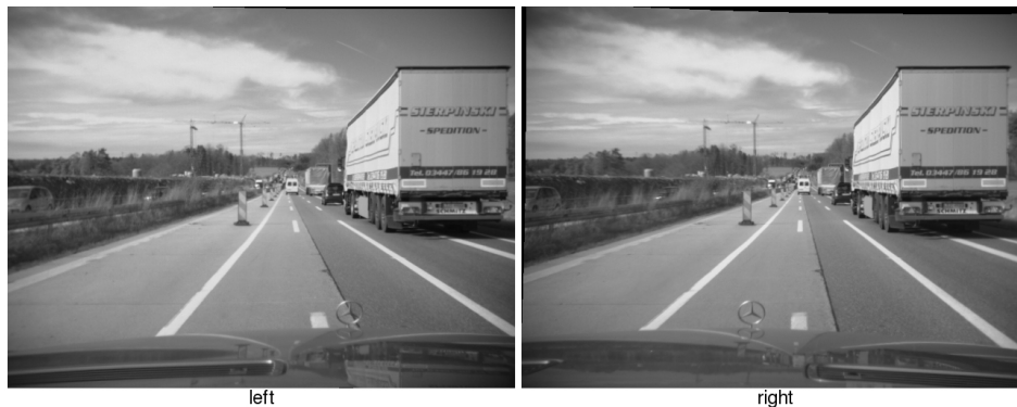
Fig. 1. A stereo pair captured by two cameras, installed on the windscreen of an ego-vehicle.
