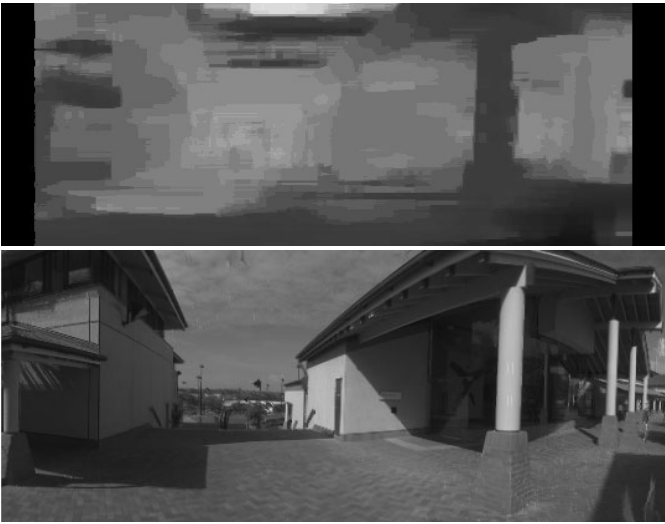
Figure 7: Range and ortho images of the reconstructed 3D scene.
