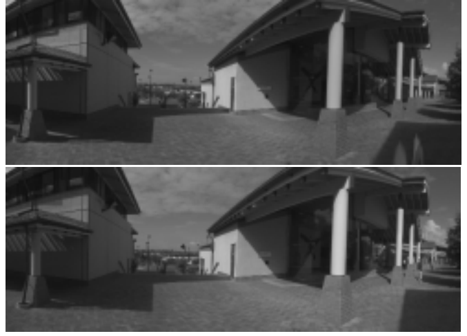
Figure 6. Stereo pair of panoramic images brought to the standard epipolar geometry by rectifying the epipolar curves.
