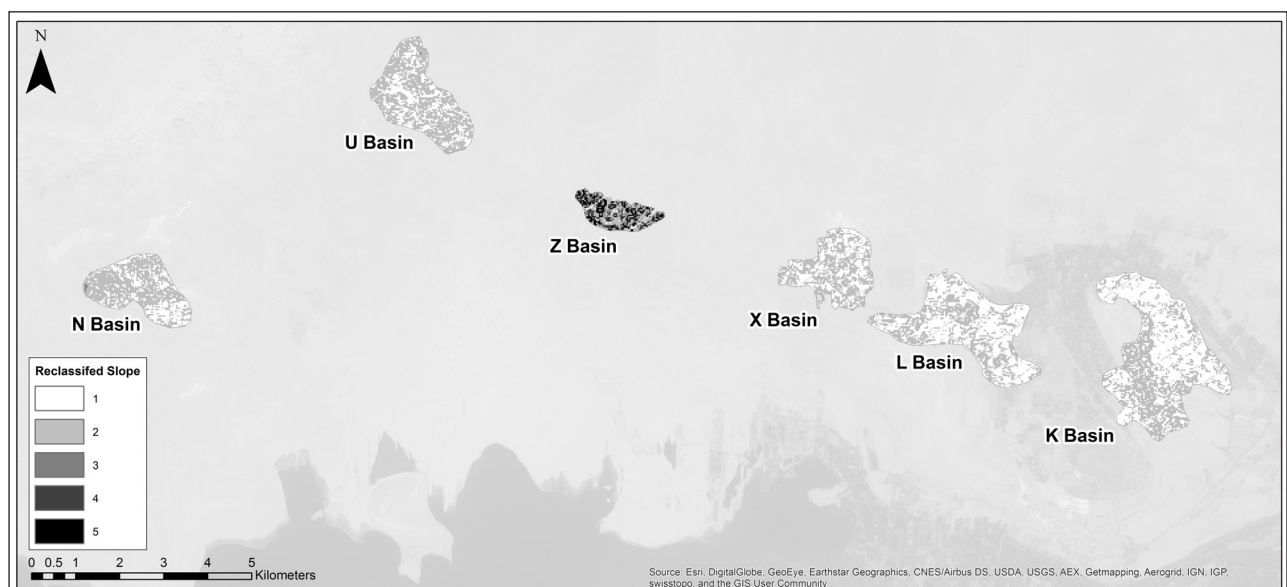
Figure 5: Reclassification of basin slope values based on the Parsons (1988) nine-unit model (see text for details).
