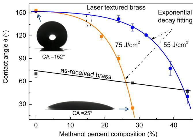
**Fig. 9.** Contact angle of methanol/water solution on unprocessed as-received brass substrate and superhydrophobic brass surfaces (left under ambient conditions for 38 days after fabrication) irradiated with 55 and 75 J/cm<sup>2</sup>.
