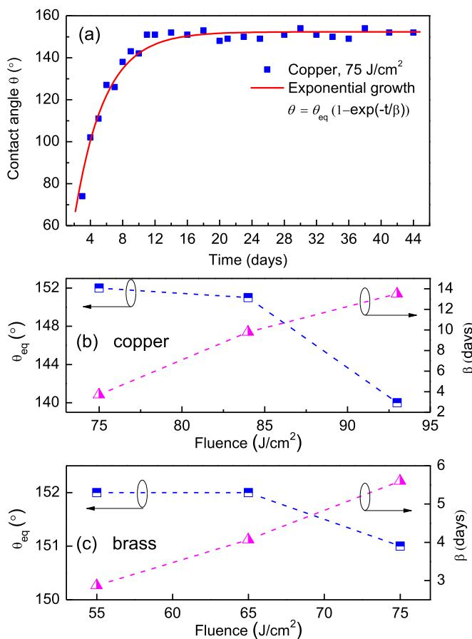
**Fig. 4.** Characteristics of the contact angle development for textured copper and brass surfaces. (a) Exponential growth behavior of contact angle over time of textured copper samples irradiated with 75 J/cm<sup>2</sup>. (b, c) Contact angle equilibrium ( $\theta_{eq}$ ) and their coefficient time constant ( $\beta$ ) as function of fluences.
