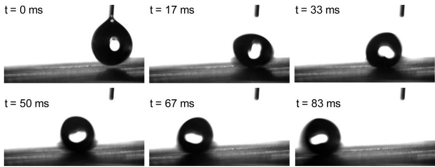
**Fig. 7.** Time sequence of a droplet rolling on a 2.9° tilted hydrophobic brass surface irradiated with 55 J/cm<sup>2</sup>.
