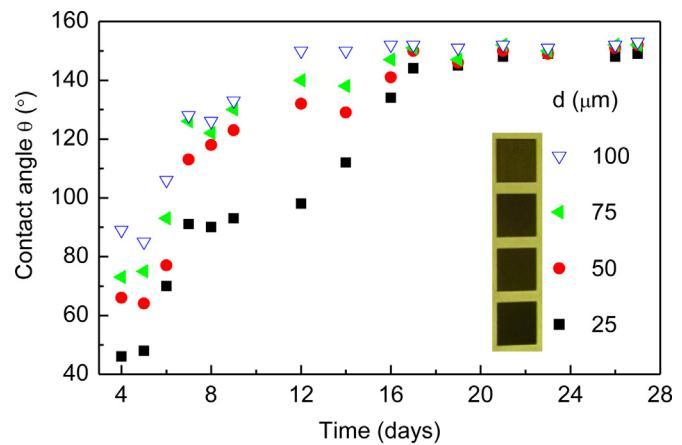
**Fig. 5.** Contact angle evolution of textured brass surfaces versus pitch size. The inset shows optical images of samples with corresponding pitch size.
