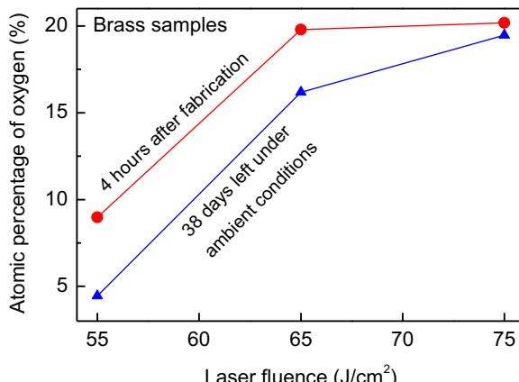
**Fig. 8.** Oxygen composition on three laser textured brass surfaces (irradiated with 55, 65 and 75 J/cm<sup>2</sup>) measured (i) directly after fabrication and (ii) after being left under ambient conditions for 38 days.
