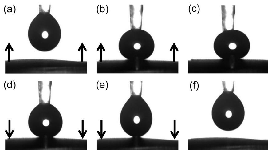
**Fig. 6.** Low adhesion between droplet and hydrophobic surface indicates small contact angle hysteresis. (a) ~5 μL water drop suspended on a syringe. (b) Strongly contacted with the lifting surface and (c) starting to slide on the surface due to the increase of upward force. (d, e) The distortion of droplet increases by lowering the surface and (f) droplet finally departed from the surface without wetting.
