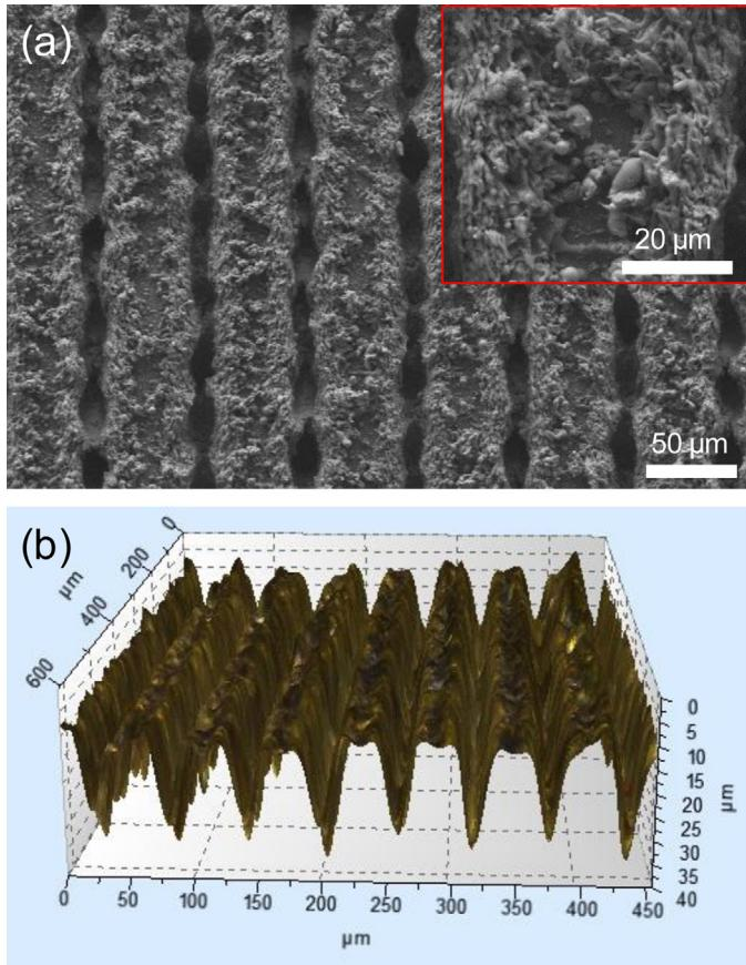
**Fig. 2.** Scanning electron microscope (SEM) and microscopy images of the laser textured brass surface irradiated with  $65 \text{ J}/\text{cm}^2$ ,  $d = 75 \mu\text{m}$ . (a) The SEM image show laser induced microgrooves. Higher magnification is presented in the inset indicating micro-/nano roughness. (b) Microscopy image obtained by focus stacking of optical images showing surface structures and depth of the microgrooves.
