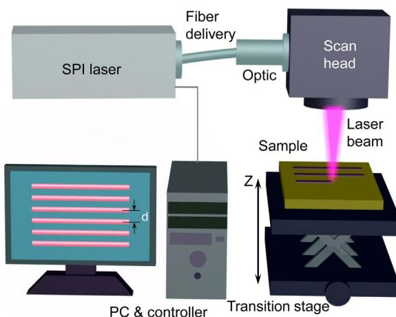
**Fig. 1.** Schematic of optical setup for fabrication of microgroove structures on copper and brass surfaces.
