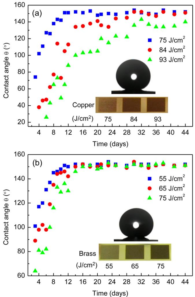
**Fig. 3.** Contact angle development over time for various fluences. (a) Copper and (b) brass surfaces. Optical images of the samples with corresponding laser fluence are shown in the insets along with images of droplets on a surface with high contact angle.
