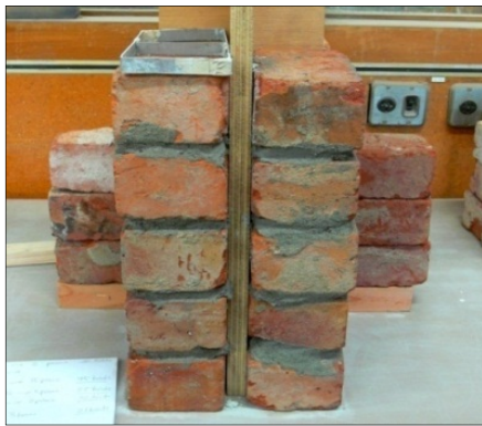
(a) Masonry prism construction against sideboard
