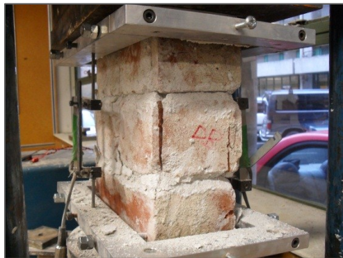
Figure 2: Prism compression test
