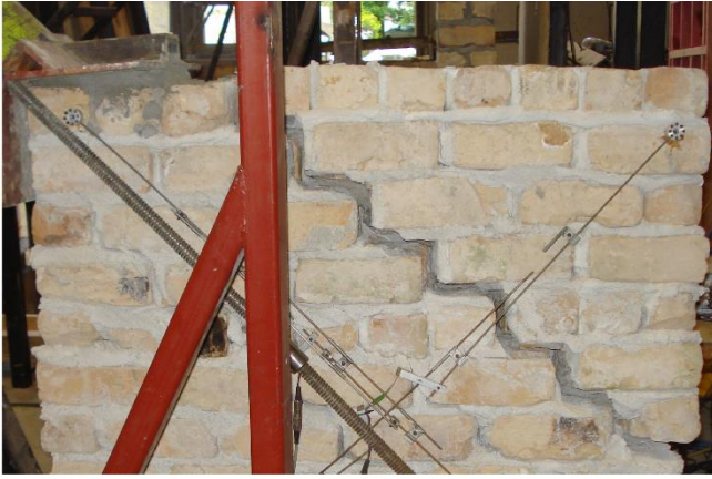
Figure 7: Diagonal crack in a wallette.
