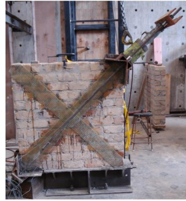
Figure 4: Test setup. For clarity, only one of the two portal gauges is shown. The other portal gauge was located behind the high-strength steel rod.
