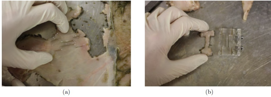
Figure 2: Sample preparation. (a) The tissue has been marked using the sample tool. (b) A surgical scalpel is then used to trace around the outside of the tissue and a repeatable sample is produced.
