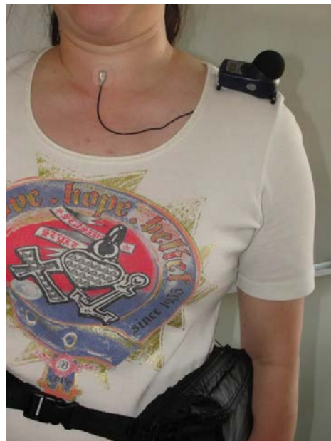
Figure 1. A person wearing the APM (ambulatory phonation monitor) attached to the neck and a noise dosimeter positioned on the shoulder.
