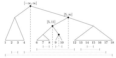
Fig. 11 Nested set of intervals represented by interval tree data structure.
