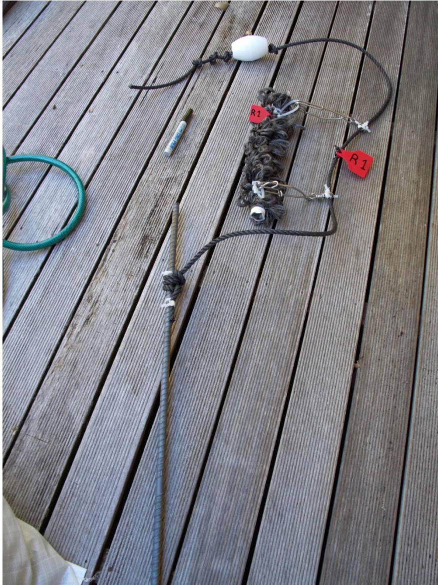
Figure 5.2 Settlement collector setup showing artificial collector (looped rope) attached by stainless steel shark clips to anchoring line which is tied to a steel rod hammered into the sediment.
