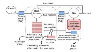
Figure 3: Data structure and architecture of CINLJ
