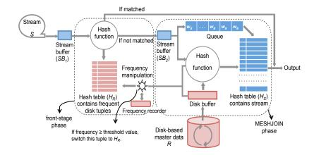
Figure 1: Data structures and architecture of CMESHJOIN
