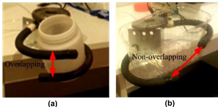
Figure 7. (a) Double fingered soft gripper was used to grip a plastic cup filled with water where overlapping is allowed and (b) Soft gripper was used to grip cuboid plastic container of greater dimension, where the distance between two fingers was adjusted and there was no overlapping.
