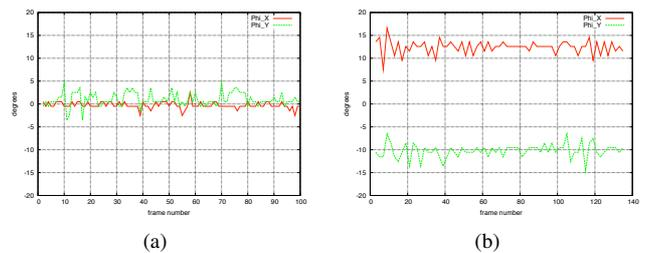
Fig. 8. Estimation of navigation angles for the (a) synthetic and (b) desktop sequence.
