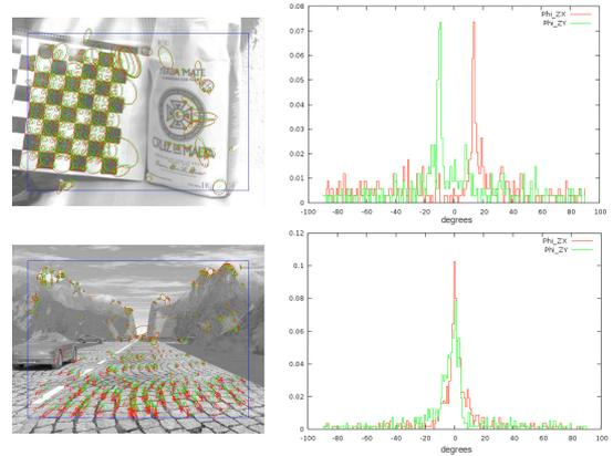
Fig. 7. Images showing tracked blobs and histograms computed for the estimation of angles  $\phi_{zx}$  (red) and  $\phi_{zy}$  (green).
