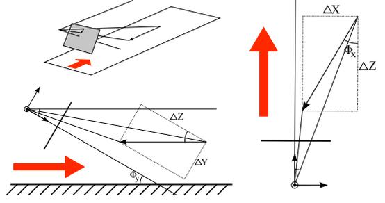
Fig. 4. A tilted camera translating along a plane (top left), motion angles (tilt) on the  $ZY$ -plane (bottom left), and on the  $ZX$ -plane (yaw; right).
