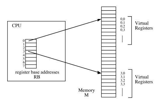
Instructions refer to main storage by adding the displacement field of 8 bits (e.g) from the instruction to a virtual register used as a base to generate the full 32-bit (e.g.) address of a 32-bit (e.g.) word. The example architecture chosen is symmetric (370-style) rather than load/store (reference to paper on relative performance of each). Load/store architectures involve some difficulties that will be discussed later.
