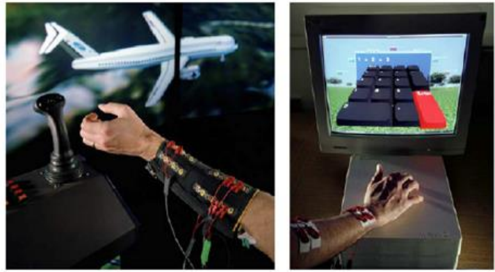
Figure 2.5: Virtual joystick based on sEMG gesture recognition [49, 50]
