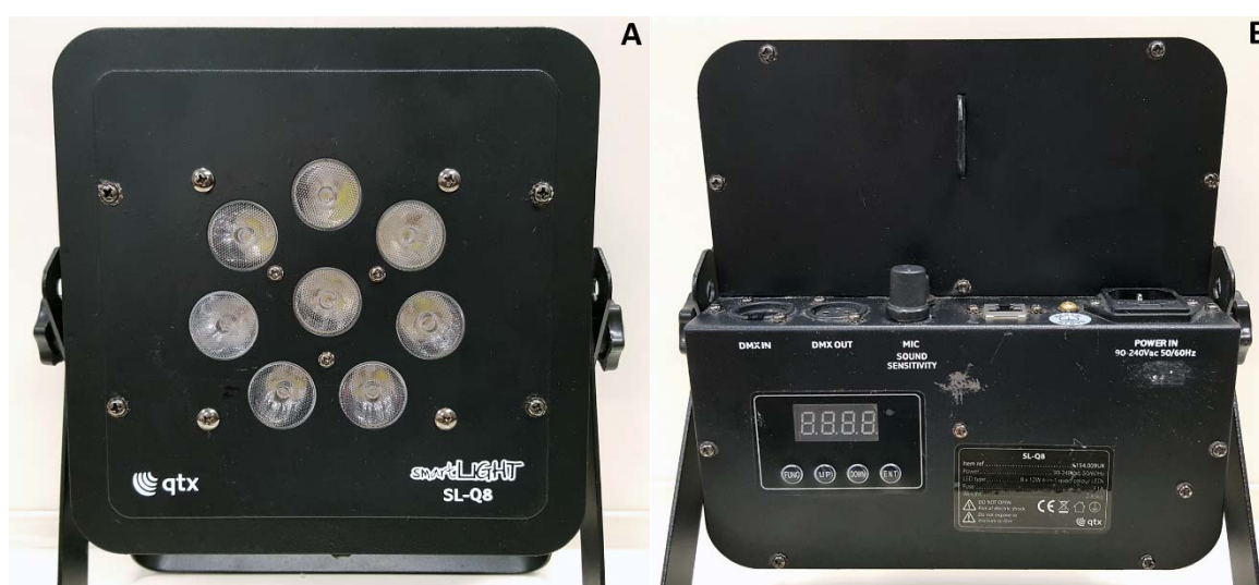
Figure 4.1. (A) Front view of the QTX SL-Q8 quad-colour RGBW-LED stage lights used to illuminate the chick experimental pens. Each of the 8 lamp units on the front panel contained a 12 W RGBW LED. (B) Rear view of the stage light showing the DMX control display and DMX input and output sockets. Each unit was assigned a starting DMX address (e.g. A001, A007, A013...) and so multiple units could be managed by one DMX controller by “daisy-chaining” successive units together with DMX cables.
