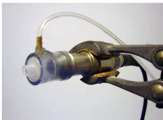
Figure 2.5. Image of the ultrasound probe with plastic stand-off attached. The inlet and silicon tube through which saline was pumped to act as a coupling fluid is shown on the superior aspect of the stand-off. The ultrasound probe was hand-held during its operation.
