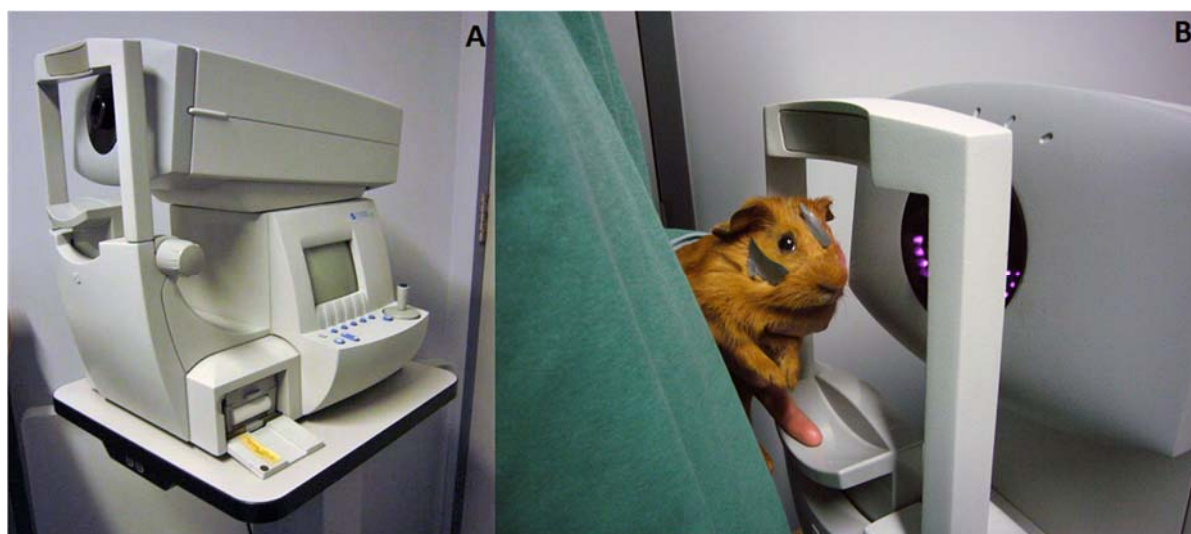
Figure 2.2. Refractive status of the guinea pigs was measured objectively with a Humphrey Autorefractor HARK-599 (A). Measurements could be made on awake hand-held guinea pigs (B). If necessary, the head was stabilised by gently holding the muzzle of the guinea pig with the other hand (not shown).
