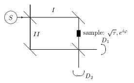
Figure 2: A particle emitted from source S impinges on the Mach-Zehnder interferometer where it can follow path I or path II. The particle can be detected in  $D_1$ , in  $D_2$ , or be absorbed in the sample.
