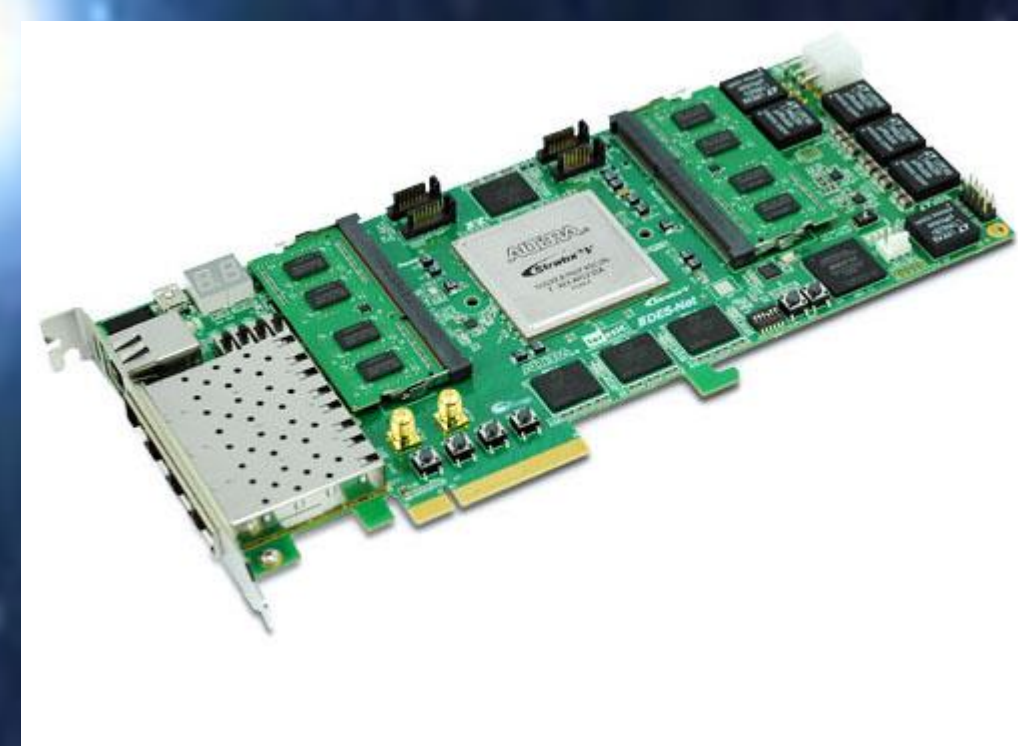
Fig 4. Terasic DE5 Board 5 with Altera Stratix V GX 7 FPGA
