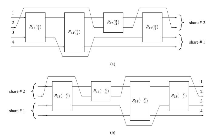
FIG. 1: Experimental realization of (a) the encoding stage of a two-component two-share configuration by an array of effectively two-dimensional beam splitters depicted as boxes. The decoding stage (b) is just the encoding stage (a) in reverse order, with inverse beam splitters.
