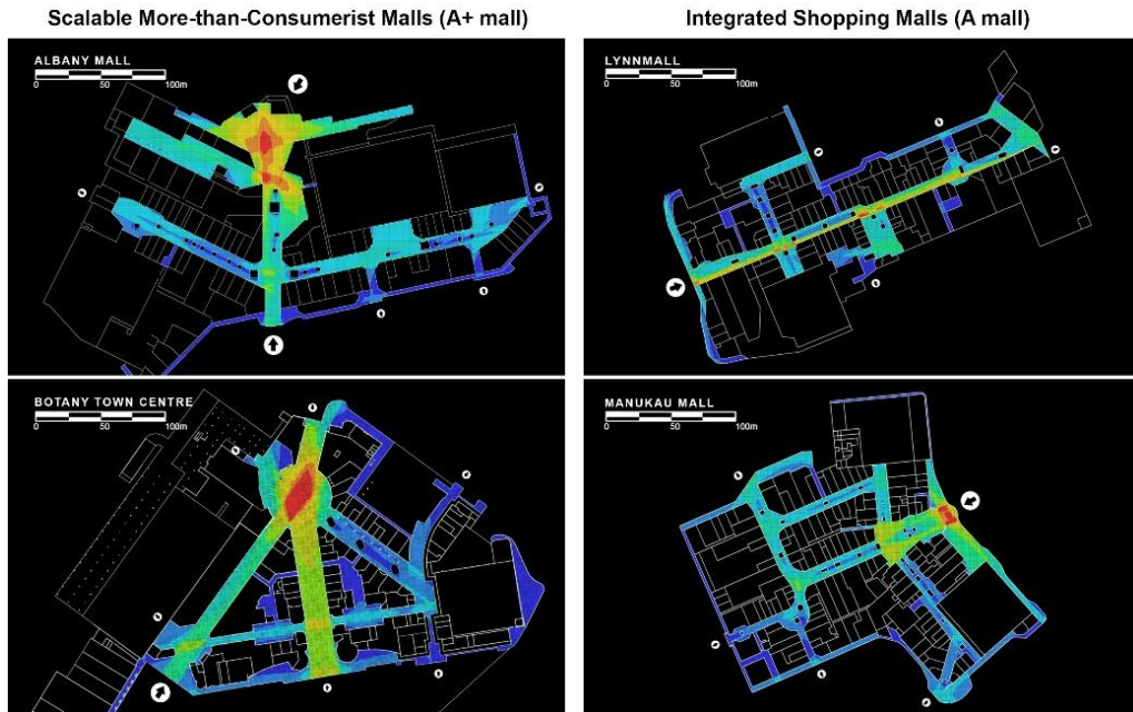
Figure 10. Visibility Graphs of the Intervisible Points Internal (Both Indoor and Outdoor) to Malls (DepthmapX)
