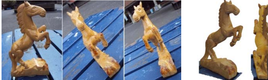
Fig. 4 Three out of 37 input images of the horse model data set (left) and the resulting reconstructed 3D model (right).
