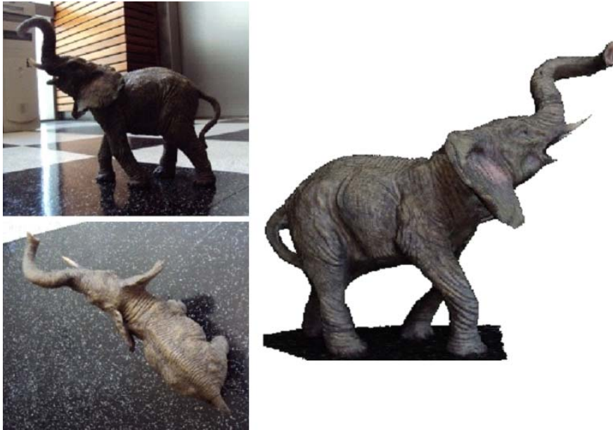
Fig. 6 Two out of 21 input images of the elephant model data set (top) and the resulting 3D reconstruction (bottom).
