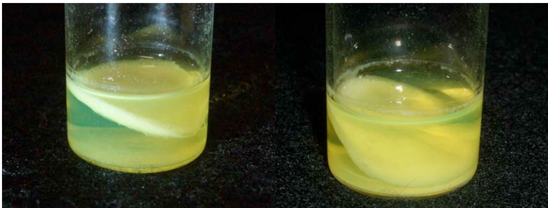
Figure 1-7: Partially collapsed mats.
